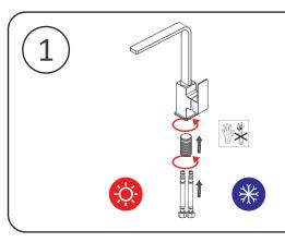
1. Install flexible hoses and the threaded tube onto the mixer, ensuring the O-ring is flat, the hoses are tight, and the threaded tube is secure.
