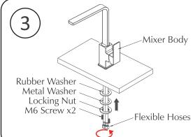
3. Install the rubber washer and metal washer over the flexible hoses and push up until it is firm against the surface being mounted on, tighten the locking nut securely with screws to ensure the mixer is firmly attached to the surface.
