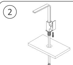
2. Put the mixer over the center of the hole to be used for mounting. Ensure the flexible hoses and threaded tube are pushed through first.
