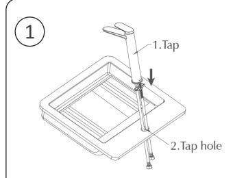
1. Leave the hoses connected to the tap, Insert the QBF and the hoses of the tap into the tap hole.
