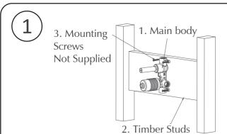
1. Place item (Main Body) onto the timber studs or concrete wall e.t.c. screw into the frame.
