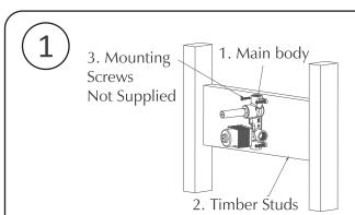
1. Place item (Main Body) onto the timber studs or concrete wall e.t.c. screw into the frame.
