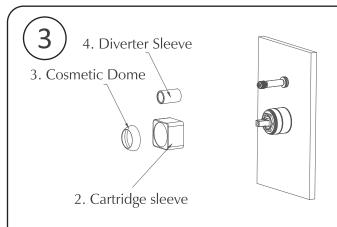
3. Install cartridge sleeve, diverter sleeve and cosmetic dome on the main body.
