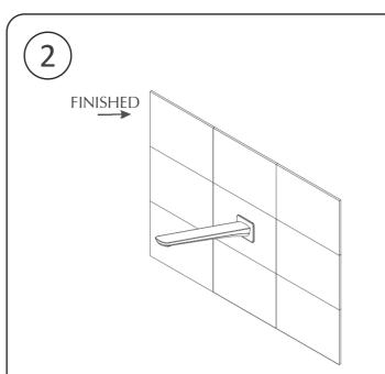
2. Turn the Spout body onto the outlet thread, and ensure the spout in the right direction.
