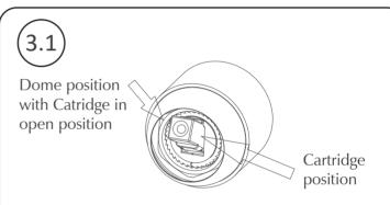
3.1. Please tilt cartridge lever to water flow open position, twist handle left and right to make sure cosmetic dome is in the right position before you tighten the handle.
