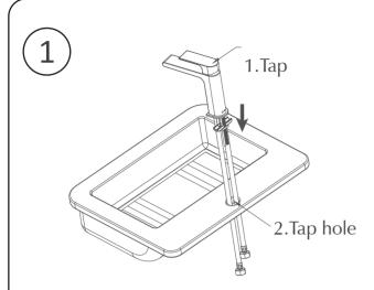
1. Leave the hoses connected to the tap, Insert the QBF and the hoses of the tap into the tap hole.
