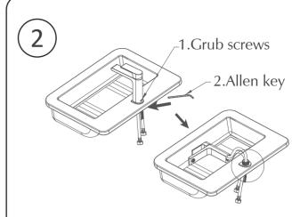
2. Loosen the grub screws to separate the tap from the QFB and rest the tap on provided cloth to avoid scratching.
