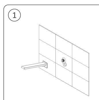
1. Wrap the Telflon tape around the G1/2 outlet thread.
