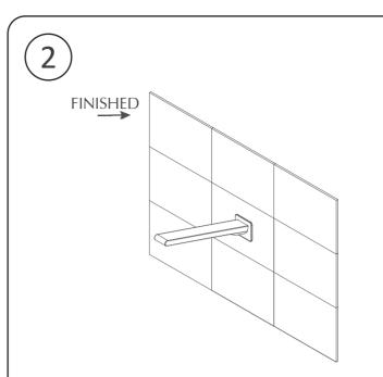
2. Turn the Spout body onto the outlet thread, and ensure the spout in the right direction.
