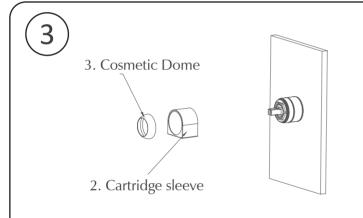
3. Install cartridge sleeve and cosmetic dome on the main body.
