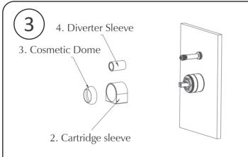
3. Install cartridge sleeve, diverter sleeve and cosmetic dome on the main body.
