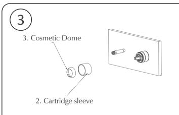
3. Install cartridge sleeve and cosmetic dome on the main body.
