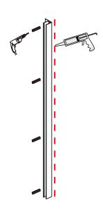
Put silicon behind channel and clean the wall before you install
