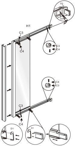
Push the D1 into the aluminum first, make sure the two little bar go into the right position.
